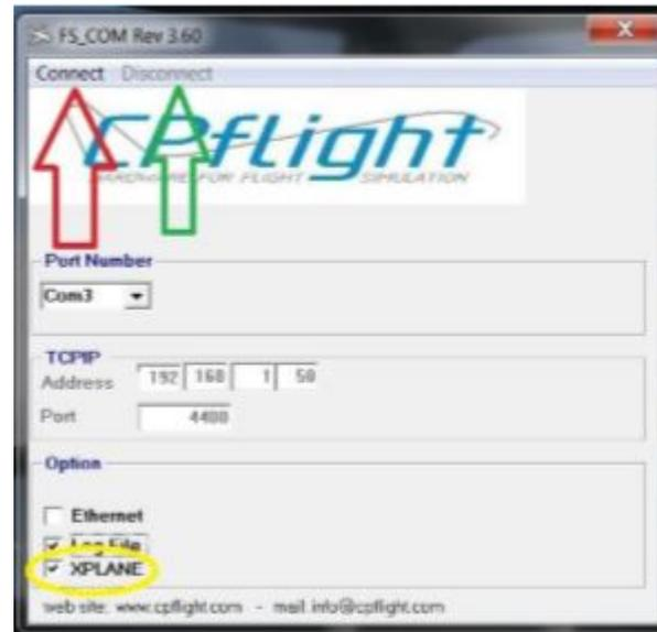
Please verify the right communication port number into the driver window ( must be the same used to test the hardware with the test utility, like showed at the begin of thuis manual).
