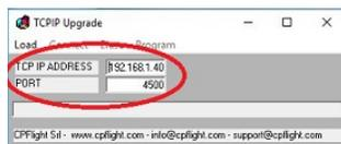
To proceed with the firmware upgrade, activating the bootloader present in the microcontroller's flash memory, you have to power the MCP pushing and holding pushed the CMDA button. Then please run the program TCPIP\_upgrade.exe and verify that the TCPIP parameters (TCPIP address and port) are the same used normally to communicate with your PC. If not please modify it into the TCP upgrade window program.
