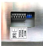
**COM:** Common pole for External A/T disengage and TO/GA
