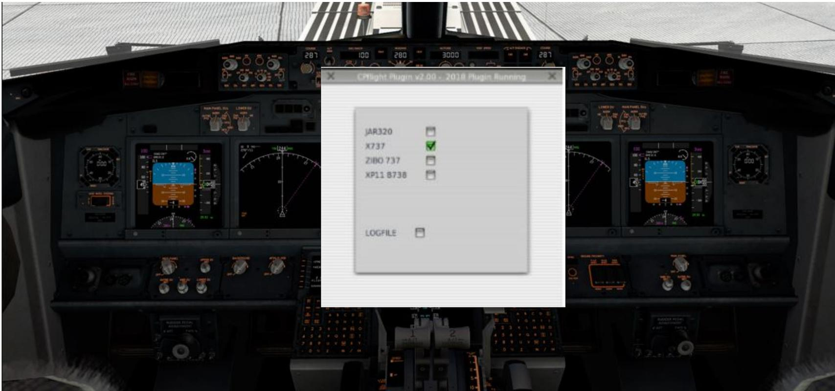
Download and install from CPflight web site the file InstXPlane11.zip and xtract the installer and run it following the instructions. Please be sure to install the driver under the plugin folder of your PC else the plugin wil not activated by XP11. So use the browse button of the installer to modify the folder if different by the default folder of the installer.
