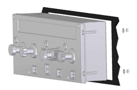
Recessed mounting on metal sheet, bracket, wood or MDF (max thickness 10mm)
