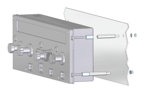
Mounting on a bottom plate. Use the spacers provided, Predispose holes for the passage of the cables.
