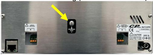
To avoid sensitivity to electrostatic discharge or other disturbances, it is good practice to connect together the FCU320 and EFIS320 ground screw. Connect all to the cockpit metal structure in a single point and connect everything to grounding.
