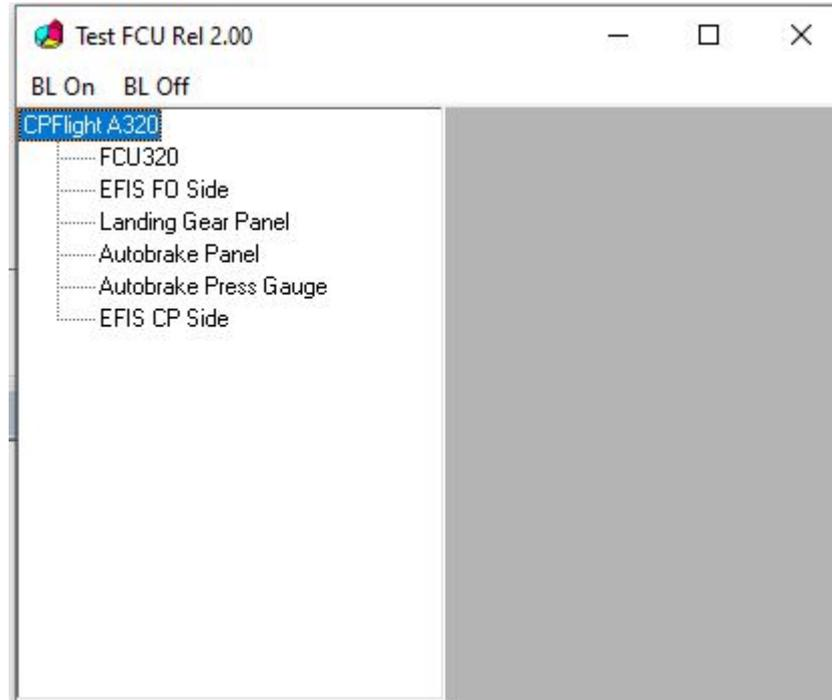
Test switches and Knobs. You will be able to see on the screen the hardware command. After this check you will be able to use the hardware with your used addon sure that the ip configuration is correct and that the hardware correctly work.
