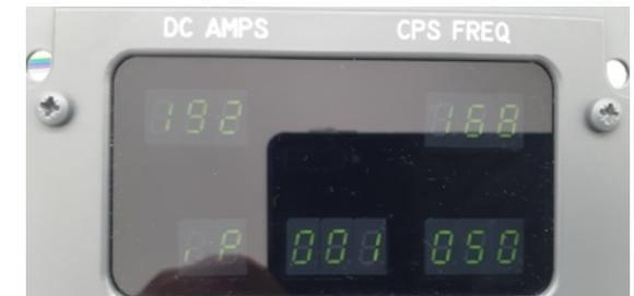
Is possible now to modify the ip number that blink. The ip values are four, with a range between 0 and 255. The first ip that will blink will be the higher byte of your ip address. So with an ip value of 192.168.1.50 the first ip parameter that will be possible to modify will be the 192, after 168 end so on....
