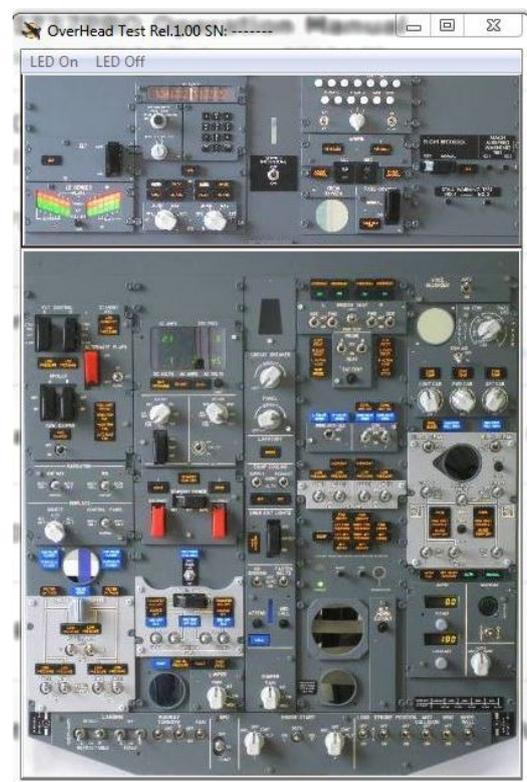
In the above figure the “TEST\_OH” utility main window. This windows allows you to select the section of the hardware for the test. Click on the FWD area to open the OVH737FWD test window
