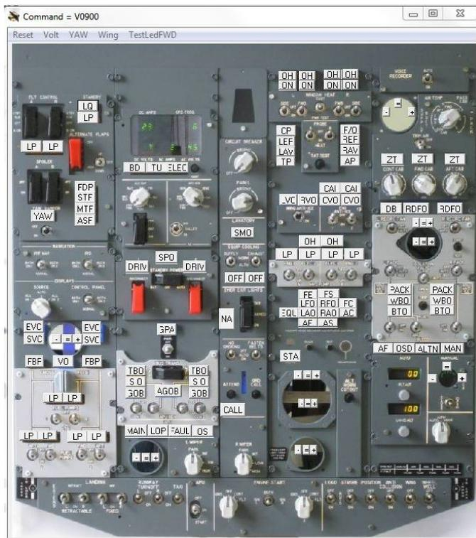
**TEST SWITCHES:** when you run the test program, all the switches (and rotary switches) positions are synchronized. The current switch position is indicated by a red text on the program window. To test a switch, move the switch hardware on the OVH737FWD panel; the text on the corresponding switch will change to indicate the new switch position.
