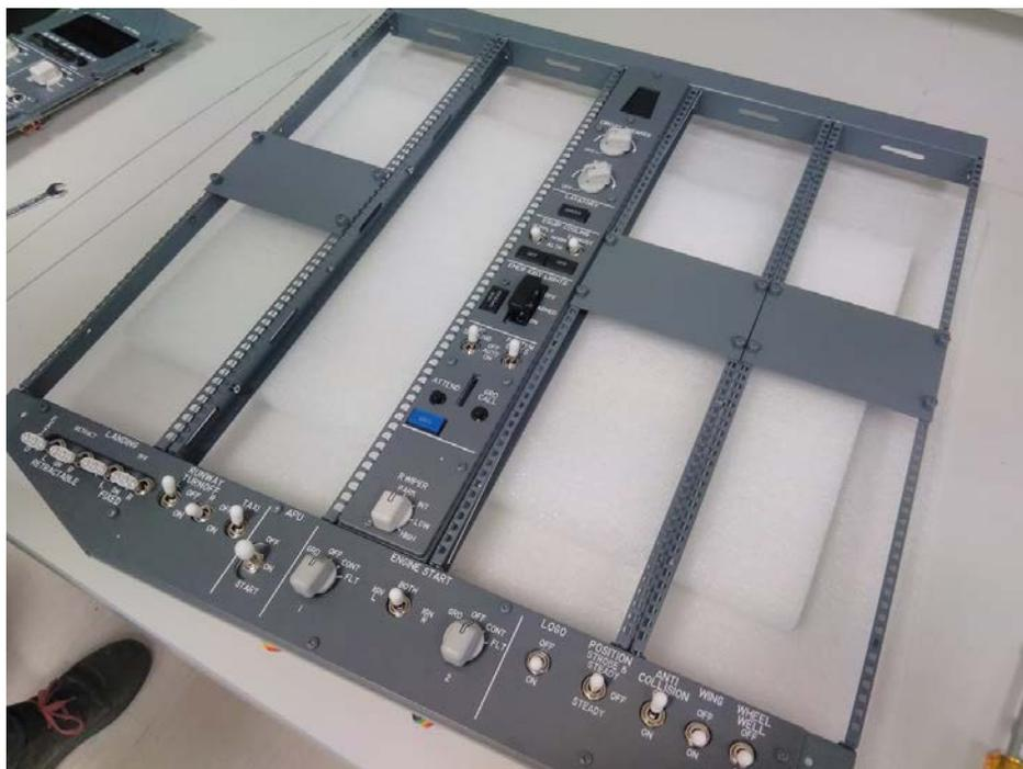
**STEP 4: FIX the ELECTRICAL panel to rails**
