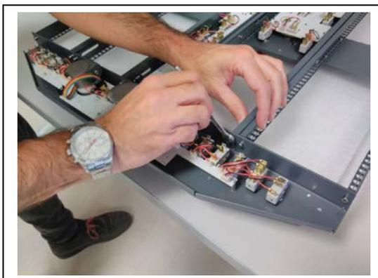
...than fix the other rail using the countersunk socket screws
