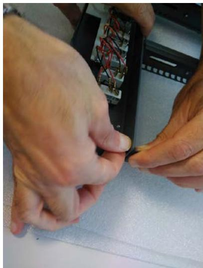
One of the landing light switches hinders the insertion of a screw (see picture below), use here the hexagon head screw.....
